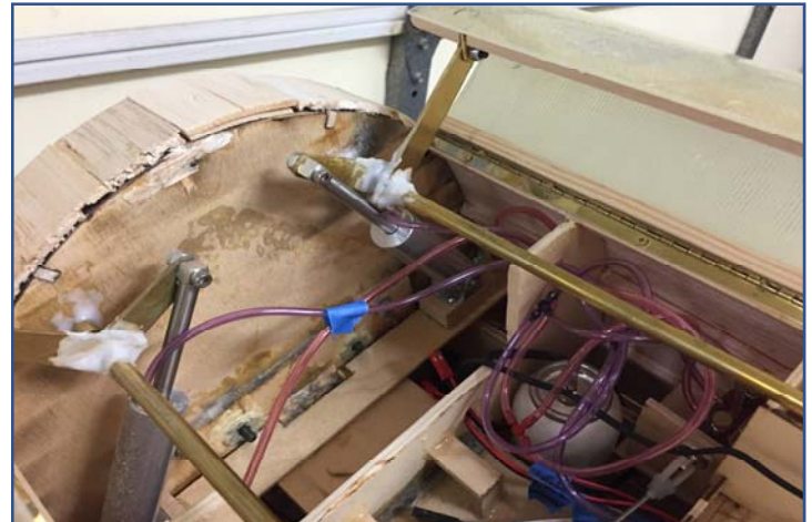
Bombay are in 4 pieces 2 on each side fasten to together with piano hinges and open and close with air cylinders.
