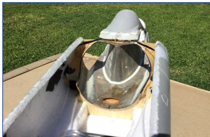
The intake is ready for paint and assembly. The oval shaped duct at the bottom will transmit low pressure forward to operate the NACA inlet ramps.
