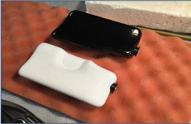
Made-to-fit, one-off, sacrificial saddle tank molds for Skyhawk. Ready to cover nearer EPS tank with black Ultracote. Will use two layers of 3.6 oz fiberglass and a little CF for layup.
