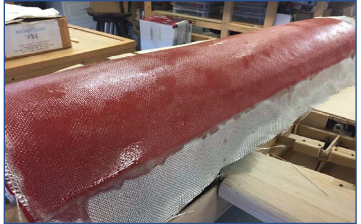
Then placed it 3 layers of 10oz fiberglass cloth and resin to make it durable, you can see the final product.
