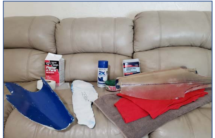
Paint the inside of mold with enamel. Wax with Turtle Wax on top of enamel for release agent
