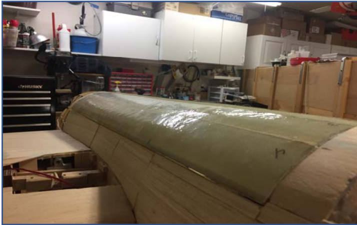
Bombay doors we're built up with balsa and ply and 1/4 spruce, and then I placed Monocote over it, waxed the Monocote with carnauba wax.
