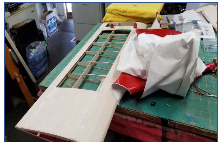
Wings have now been peeled again and will be recovered with Stitts.
