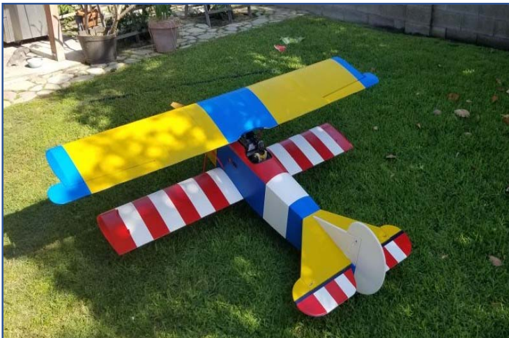
Tim Carden's Hangar 9 Fokker DVII. Peeled and recovered with Oratex. Painted with Poly Tone (Stitts) and apparently there has been a change in the formula for Oratex.
