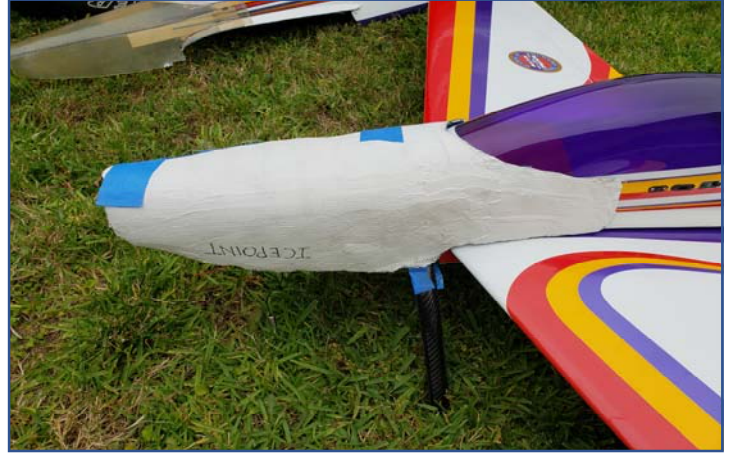
Using the good plane as a mold reference. Cover with plastic wrap
