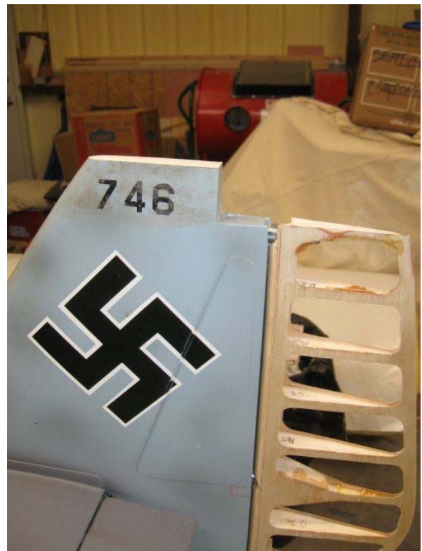
Rudder and stab cleaned up to accept new balsa tops.
