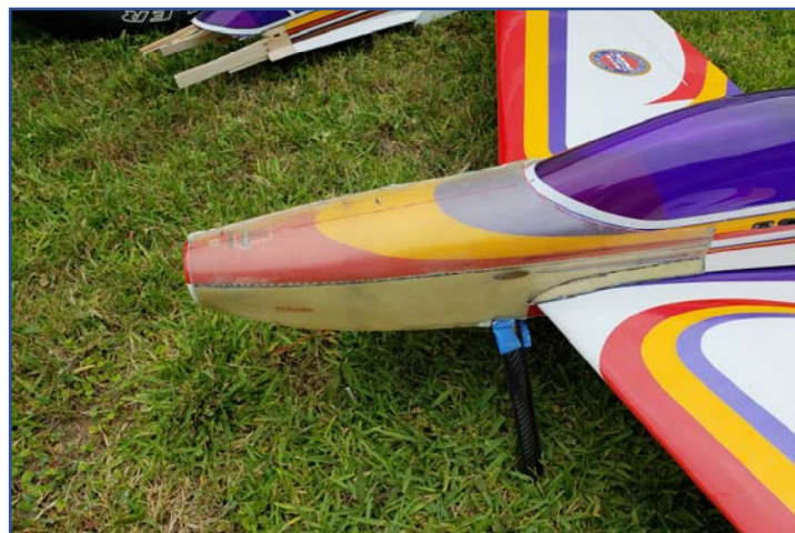
Use polyester resin and two layers of glass cloth. Sand after drying to allow for adhesion of third layer of fiberglass cloth
