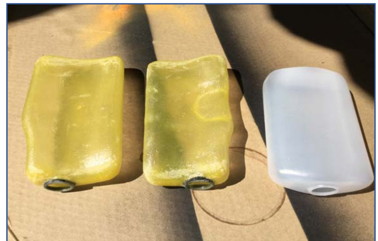
After scuffing and adding another layer of glass, the tanks are air tight. The resin was thickened with Aerosil and slathered into the cloth. The tanks each weigh 18% less than an 8oz Sullivan tank.
