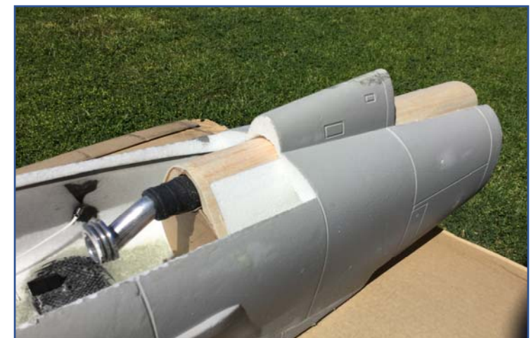
This is an eps and balsa thrust tube mold In the works. The tuned pipe is narrower than the root of the dorsal fin and will be mounted partially in the dorsal fin. The pipe will still have ventilation while leaving the thrust tube mostly unobstructed.
